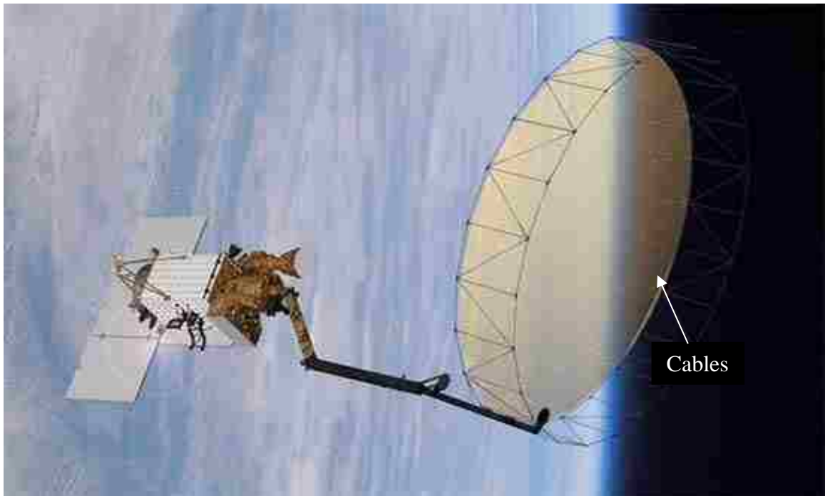
Figure 1.1.2 AstroMesh deployable satellite reflector (Northrop Grumman Corporation)
