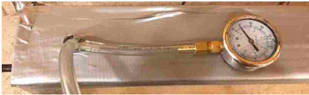
Figure 3.4.4.4 Connection between pressure gauge and chamber
