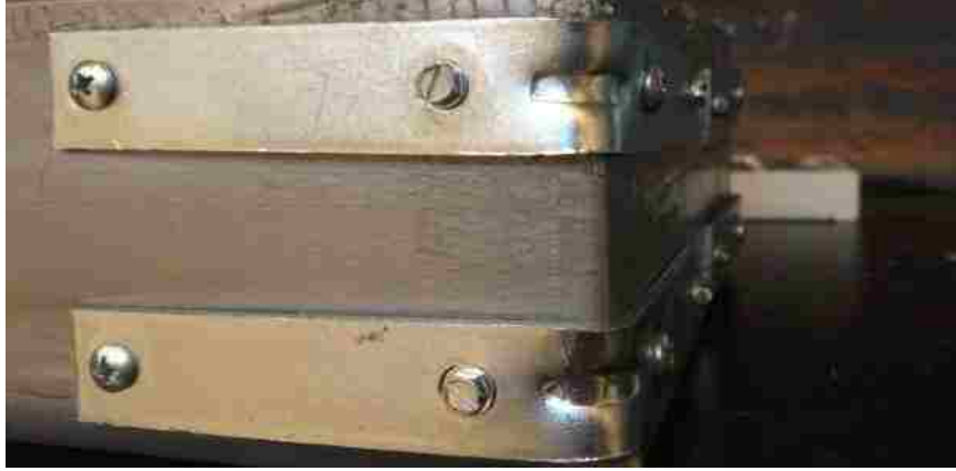
Figure 3.4.5.2 Details of the stiffened frame corners
